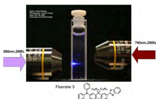
Figure 1: A fluorene dye is excited in single-photon absorption (left) and two-photon absorption (right). Note that the single-photon absorption takes place over the entire volume accessed by the beam, while the two-photon absorption is confined to the focal volume. 2
