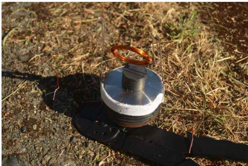
Completed motor showing the magnet coil placed just above the neodymium magnet.
