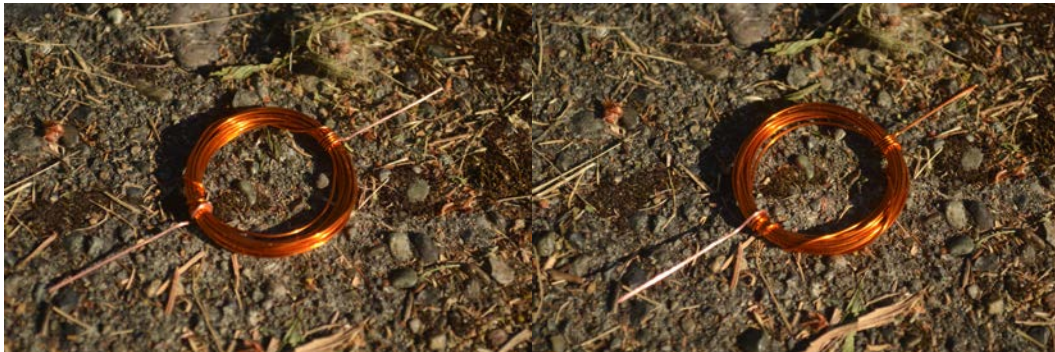
Left: top side of magnet coil, both of the arms on opposite ends have insulation sanded off.
